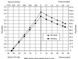
num [in.Hg] 2660 Series Base Model Flow Curve
